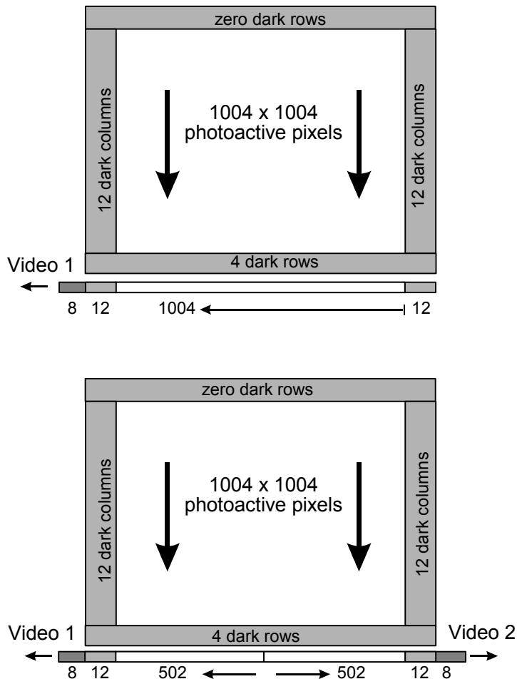
The KAI-1020 is designed to read the image out of one output at 30 frames/second or two outputs at 48 frames/second. In the dual output mode the right half of the horizontal shift register reverses its direction of charge transfer. The left half of the image is read out of video 1 and the right half of the image is read out of video 2.
