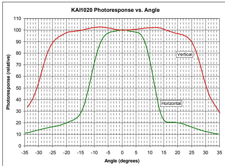
The horizontal curve is where the incident light angle is varied in a plane parallel to the HCCD.
