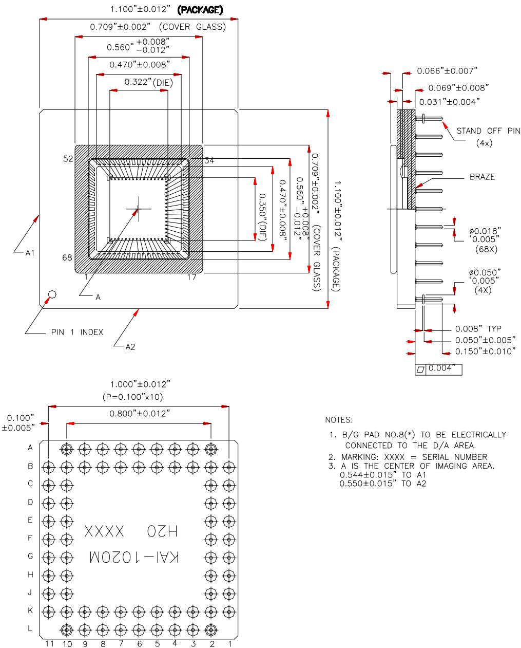
When viewed from the top with the pin 1 index to the upper left, the center of the photoactive pixel array is offset 0.006" above the physical center of the package. The pin 1 index is located in the corner
