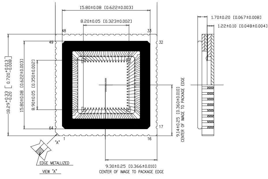
DIE ATTACH AREA SHALL BE CONNECTED TO PIN No.8.
