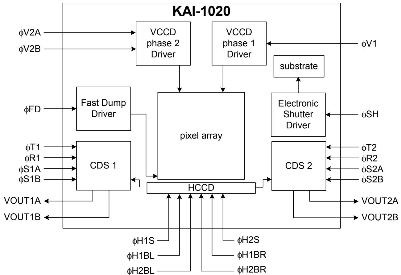
All timing inputs are driven by 5V logic. The image sensor has integrated clock drivers to generate the proper voltages for the internal CCD gates. There are two VCCD clock drivers. Both the phase 1 and phase 2 VCCD drivers control the shifting of charge through the VCCD. The phase 2 driver also controls the transfer of charge from the photodiodes to the VCCD.
