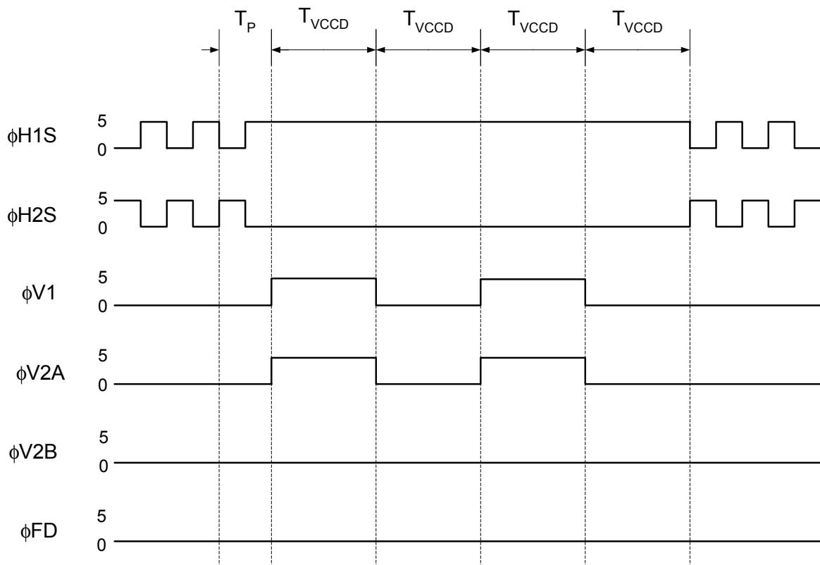
When binning two rows together only 504 rows need to be read out of the HCCD instead of the normal 1008 rows. The HCCD will hold up to two VCCD rows of full signal without blooming. Binning more than two rows may cause horizontal blooming for saturated signal levels.
