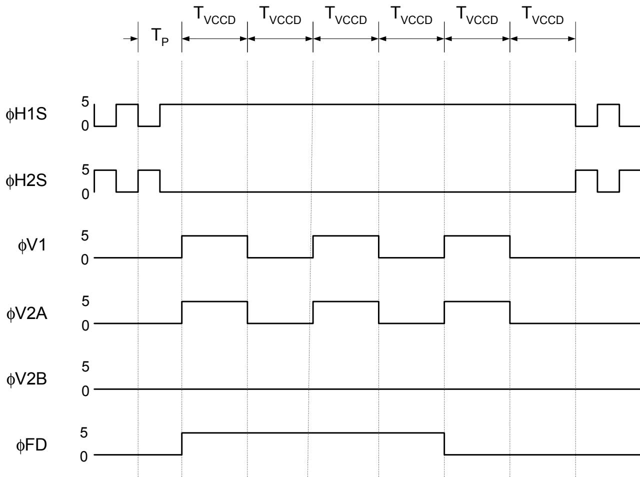
This timing diagram shows how two lines are dumped and the third is read out.  $\phi FD$  should go high once the last pixel of the preceding line has been read out. Cycle the VCCD for the number of rows to be dumped. The above timing diagrams shows two rows being dumped. When the proper number of rows have been dumped bring  $\phi FD$  low. Then clock the VCCD through one more cycle to shift a row into the HCCD.
