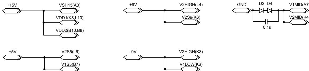
The V1MID and V2MID connections must be set to  $-1.0$  to  $-1.5V$ . Since V1MID and V2MID only sink current, two diodes can be used to set this voltage.
